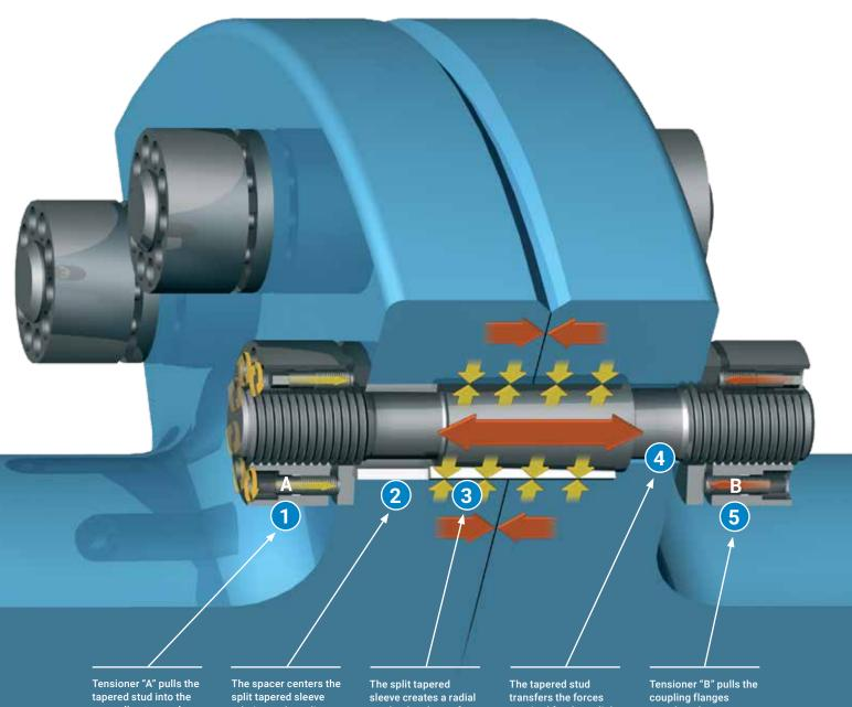
expanding tapered sleeve which is split, thus generating a radial force.
