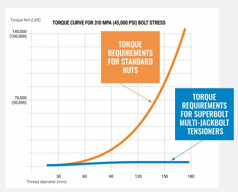
The chart shows how Superbolt tensioners remain easy to install, even on larger sizes, compared to standard hex nuts. Only hand tools are required to tighten any diameter stud/bolt.
