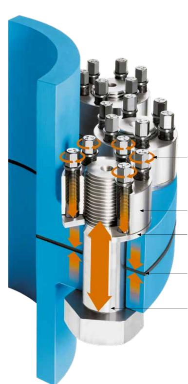
Superbolt tensioners are designed as direct replacements for conventional nuts and bolts. These devices can be threaded onto a new or existing bolt, stud, threaded rod or shaft. The main thread serves to position the tensioner on the bolt or stud against the hardened washer and the load-bearing surface.
