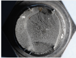
Fatigue failure (stress point nut)
