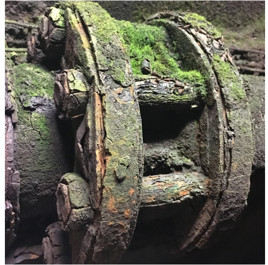
Example of extreme corrosion on a flanged connection.
