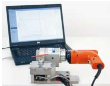
The Junker test: a joint is mounted on a test rig and exposed to a simulated vibration at a right angle to the joint. The result is displayed on the computer screen.
