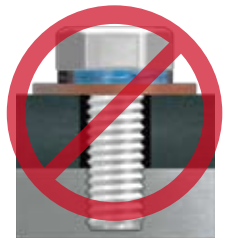
5. Nord-Lock washers must not be placed on a washer which is free to rotate.
