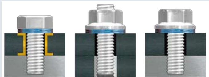
1. By using a bushing, a higher preload can be utilised and the composite material is relieved from most stress and the contact surface becomes suitable for serrated washers.
