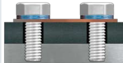
4. In order to distribute load and protect a sensitive surface, a metal washer covering multiple holes can be used.
