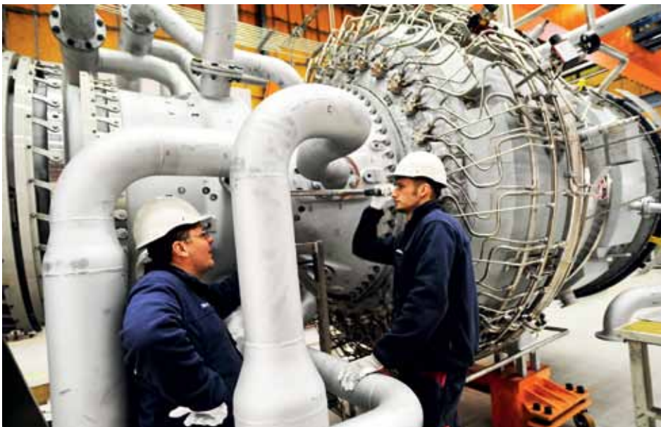
Nicklas Lundbom (left) and Oskar Gunnarsson tightening turbine joints. Siemens turbine factory in Finspång, Sweden, relies on Nord-Lock safety washers to make sure the bolts in the turbines stay put.
