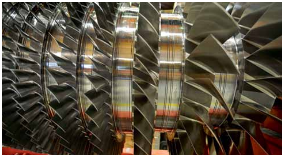
Steam and gas turbines are assembled from pre-machined steel parts. They operate in solar plants, biomass, and in oil and gas facilities, under enormous pressures and temperatures to generate electricity.
