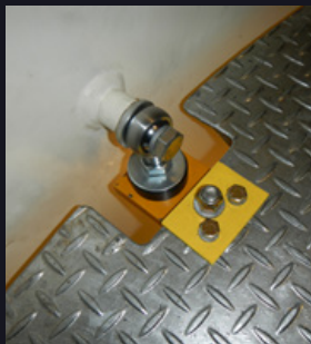
Figure 1 Actual installation on the Yaw deck of an operating wind turbine. The Nord-Lock original washers on each of the bolts help mitigate any problems due to stress and vibration.
