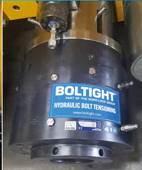
1500 Bar Hoses attached to hydraulic intensifier to activate hydraulic bolt tensioners
