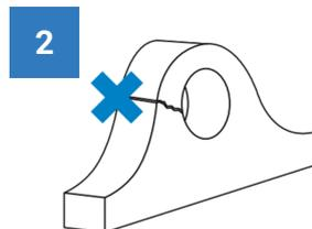
Repair any structural damage i.e. cracks or bent lug ears before installation.
