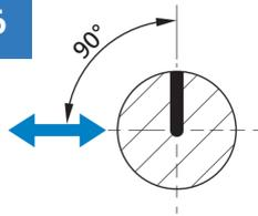
**NOTE!** If applicable: position greasing outlet 90 degrees to force direction to minimize stress concentration at outlet.
