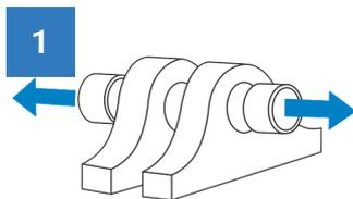
Remove any bushings to eliminate future wear between the bushing and the mounting lug.
