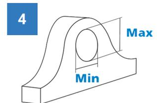
The difference between min and max diameter in the worn lugs must be within .06" (1.5 mm) for the sleeves to fit correctly.
