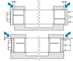
Grease the pivot (if applicable). After initial torque, move the machine through full range of motion several times and recheck torque. Check the torque after 10 hours, 40 hours and at regular service intervals to ensure proper seating of the sleeves.
