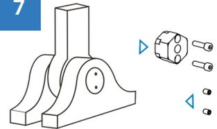
Remove the allen key screws and mounting tool. Mount the stop screws.
