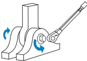
To dismount the Expander System, unscrew the fasteners on both sides and remove the washers.
