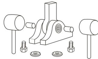
Tap the axle alternatively on left and right side until the tension on the sleeves is released (use a piece of pipe between the axle and the mallet/hammer not to damage the threads). Remove the sleeves and axle. Do not damage the threads.
