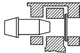
The spacer is always positioned on the opposite side of the stepped part of the axle. If the pivot already has a spacer, leave it in its position. If the Expander System includes a spacer, place it between the inner sphere of the bearing and the lug ear, with the bevel facing the bearing.
