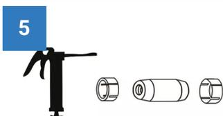
Grease the sleeves and axle with grease available, preferably graphite grease. Do not grease the threads!
