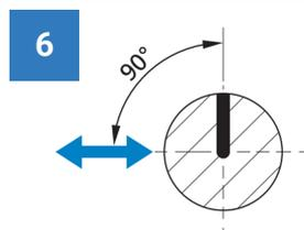
**NOTE!** If applicable: position greasing outlet 90 degrees to force direction to minimize stress concentration at outlet.
