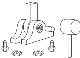
Unscrew the fasteners on both sides and remove the washers. Tap the axel end with small diameter until the tension on the sleeves is released. Use a piece of pipe between the axle and the mallet/hammer not to damage the threads.
