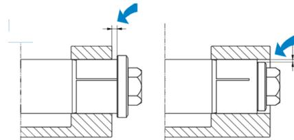
Ensure that there is a minimum distance of 0,5 mm (0.02") between the washer and the lug. **NOTE!** If flange design for easy removal of the sleeve is used there should be a minimum distance of 6 mm.
