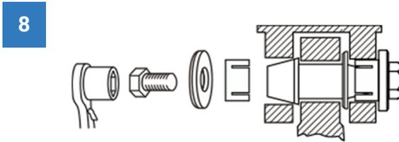
Install sleeve, washer and fastener on the side with large axle diameter. Tighten the fastener with recommended torque.
