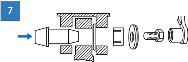
Insert the axle. Install the sleeve, washer and fastener on the side with small axle diameter. Press on the axle end with large diameter until the axial play is eliminated. Tighten the fastener with recommended torque.
