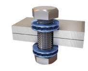
Place one pair of Nord-Lock washers underneath the head of the bolt and mount it in the through hole. Place the second pair of washers on the bolt and mount the nut.
