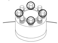
At 100% target torque, tighten the same (4) iackbolts on all studs.
