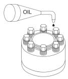
As the equipment is cooling down (around 300°F), apply penetrating oil to the jackbolts and washer and let sit for several hours. Thoroughly "wet-down" all components and re-apply during equipment cool-down period. If the tensioner is inverted, squirt oil in the gap between the nut body and the washer. Synthetic oil can be used for oiling above 300°F.
