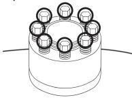
At 100% target torque, tighten all jackbolts in a circular pattern. Do this procedure for all studs (1 round only). See Helpful Tip #6 on page four.
