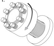
Lubricate the thread of the main stud and slide the hardened washer onto the stud. Spin the tensioner onto the thread until it seats against the washer. Then back the tensioner off to provide a small gap between the nut body and the washer.
