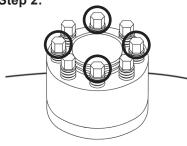
Tighten (4) jackbolts at 90° apart on all studs with a partial torque of approximately 50% (this serves to seat the flange). If using an air impact, use a reduced setting or lightly pulse the trigger.
